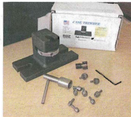
The RDZ Case Trimmer sets up on a drill press and makes quick work of piles of brass. If there is a downside to the product it is that cases must be unprimed when they are trimmed.
